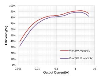
Figure 2.Efficiency vs Load Current, Vin=24V
