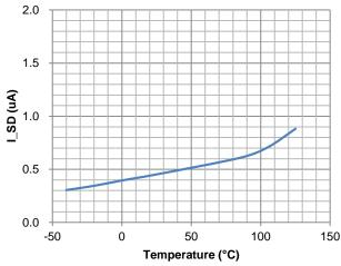
Figure 3. Shut-down Current vs Temperature
