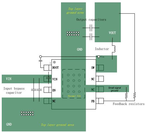
Figure 18. PCB Layout Example
