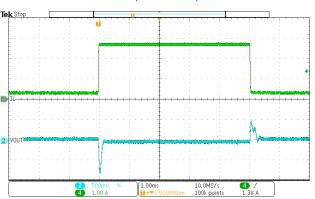
Figure 17. Load Transient VOUT=5V, IOUT=0.3A to 2.7A, SR=250mA/us
