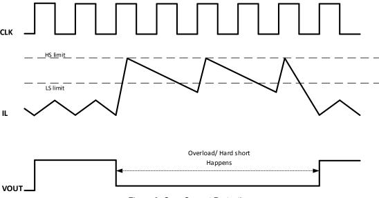
Figure 9. Over Current Protection
