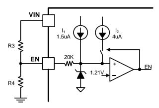
Figure 8. Adjustable VIN UVLO
