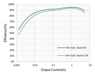
Figure 1.Efficiency vs Load Current, Vin=12V
