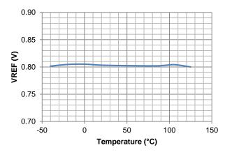
Figure 5. Reference Voltage vs Temperature
