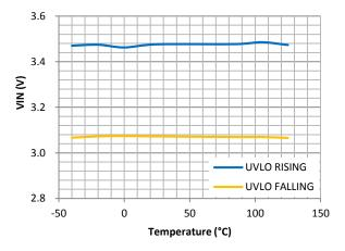
Figure 6. VIN UVLO vs Temperature
