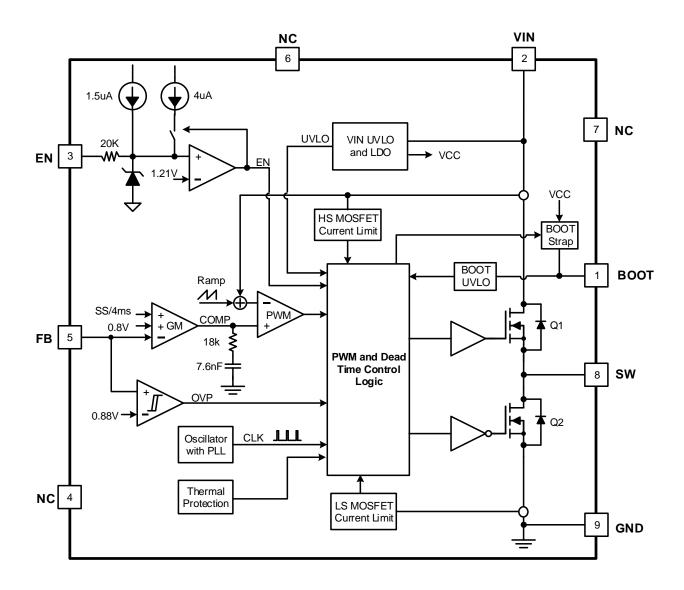
Figure 7. Functional Block Diagram
