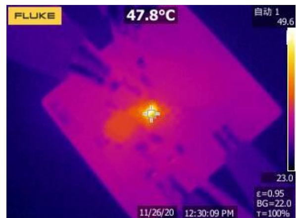
Figure 23. Thermal, 24VIN, 5Vout, 0.6A
