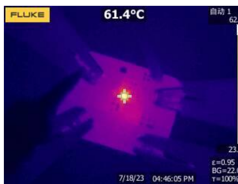
Figure 20. Thermal, V_{IN}=5V , V_{OUT}=1.2V , I_{LOAD}=3A
