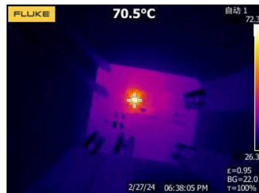
Figure 29. Thermal, 24VIN, 5VOUT, 0.8A
