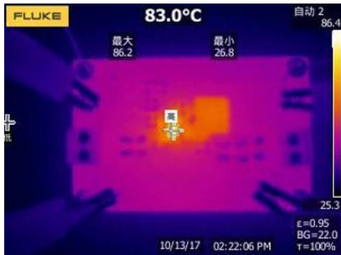
Figure 10. Infrared Thermal Image, Iout=2A
