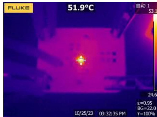
Figure 20. Thermal, V_{IN}=5V, V_{OUT}=1.2V, I_O=2A
